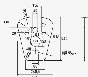
FLUSH FERRAGENS PARA CISTERNAS CISTERN MECHANISM
